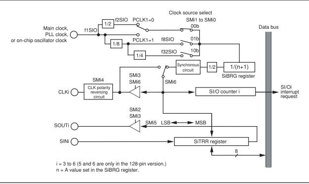
Figure 14.36 SI/Oi Block Diagram
